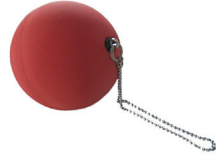
sphericle weight with ballchain and soother dummy according to EN 12227-2
